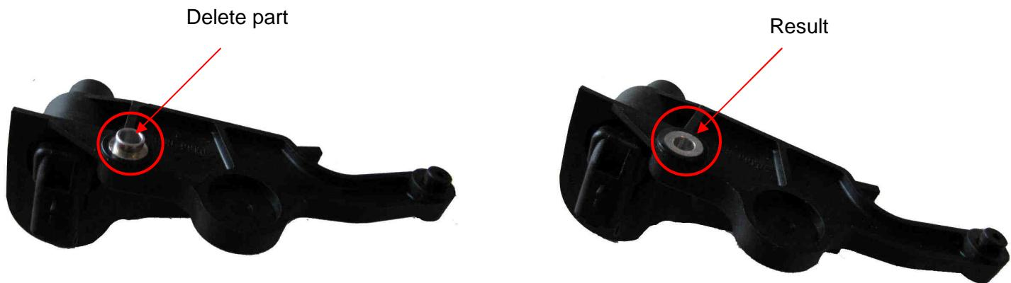
Then drill the insert at  **$\varnothing 7.5\text{mm}$**  in order have a tuning clearance.
